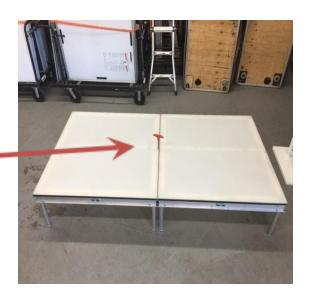
4. Place side panels on each side of the stages but leave and opening in the back so you can put lights underneath.
